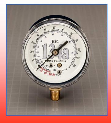
Gauges are calibrated so that zero on the gauge indicates atmospheric pressure (14.7 psia). This compound gauge also allows vacuum readings (pressures that are below atmospheric) expressed as in. Hg.
