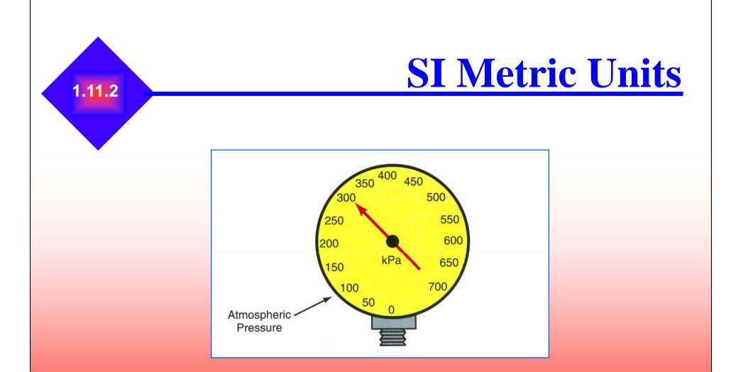
In SI units, atmospheric pressures are expressed in kPa (kilopascals). Normal atmospheric pressure is 101.3 kPa, but gauges are often calibrated at 100 kPa for atmospheric pressure for ease of use.
